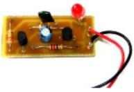
Here we will make LED flashers which have wide application to real-world life, including alarms that go off and on a repeated amount of times, sirens such as from a police car flashing on and off, and many other various units.
